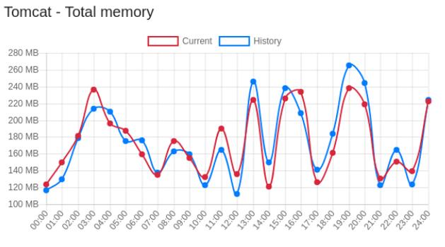
**Figure 1: Memory consumption of a Tomcat instance**
